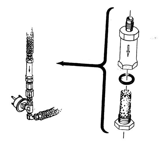
REMOVE OIL FILTER FROM LINE AND DISSASSEMBLE UNIT. WASH PARTS WITH SOLVENT AND BACK FLUSH THE BRONZE ELEMENT. CHECK CONDITION OF "O" RING AND REPLACE IF NECESSARY. REASSEMBLE UNIT AND INSTALL FILTER IN THE TURBO OIL SYSTEM. CLEAN FILTER AT EACH OIL CHANGE.
