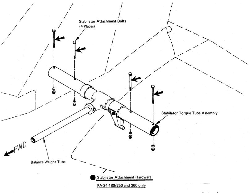
Bolt AN174-C32A P/N 502 329 (Corrosion Resistant) or Bolt AN174-32A P/N 402 329 (Non-Corrosion Resistant) Washer AN960-416L P/N 407 585 Nut MS20365-428C P/N 404 888
