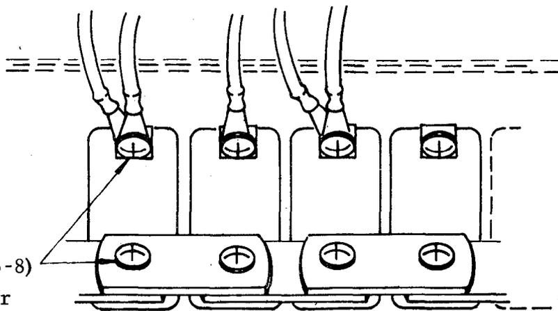
Lock Washer - (AN935-8) must be installed under screw head at each circuit breaker terminal.
