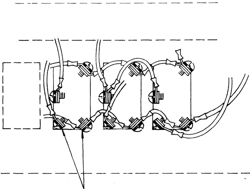
Lock Washer (AN936-A6) must be installed under screw head on each switch terminal.
