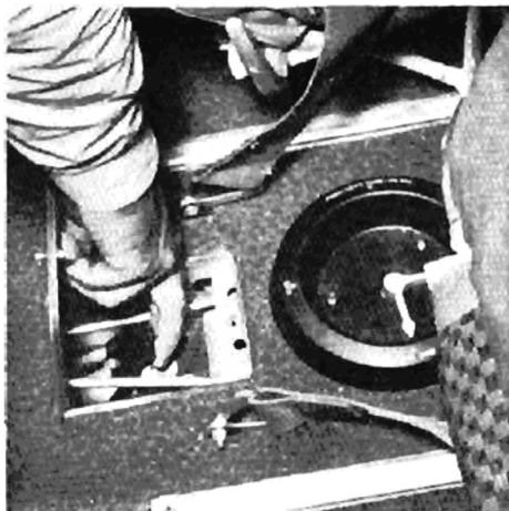
Two rubber like fuel cells in the inboard leading edge sections of the wings provide fuel capacity. Available as optional equipment on the PA-21-250 only are two auxiliary fuel cells located outboard of the main fuel cells. Auxiliary fuel cells have a 15 gallon capacity. The cells should be kept full of fuel during storage of the airplane to prevent accumulation of
