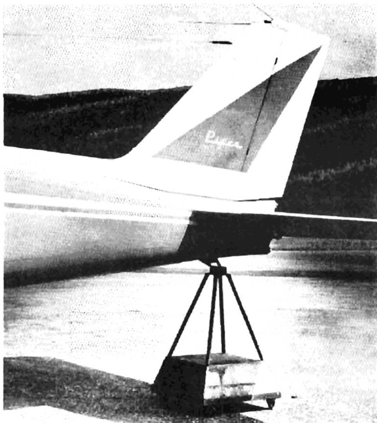
jacks and a tail support. Approximately 300 lbs. of ballast should be placed on the base of the tail support before jacking up the airplane.
